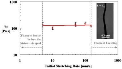
**Fig. 8** Extensional viscosity ( $\eta_{\rm E}$ ) derived from Eq. 1 for 0.3% treated CNT suspension as a function of the initial stretching rate. Each *open square* represents the average value from four separate runs of
