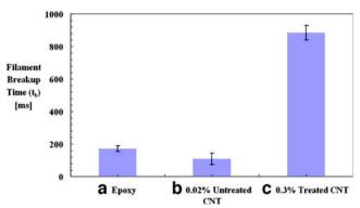
**Fig. 6** Filament breakup time ( $t_b$ ) for **a** epoxy, **b** 0.02% untreated CNT suspension and **c** 0.3% treated CNT suspension. Stretching rate= 100 mm/s and endplate displacements=3 mm from starting positions
