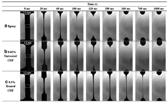
**Fig. 3** Sequence of images showing the extensional deformation for the filaments of **a** epoxy, **b** 0.02% untreated CNT suspension and **c** 0.3% treated CNT suspension. Stretching rate=100 mm/s; endplate
