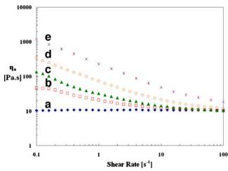
**Fig. 5** Apparent steady shear viscosity ( $\eta_a$ ) of **a** epoxy, **b** 0.05%, **c** 0.1%, **d** 0.25% and **e** 0.5% untreated CNT suspensions, showing significant viscosity enhancement at relatively low CNT concentration levels
