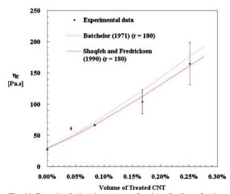
Fig. 11 Extensional viscosity ( $\eta_{\rm E}$ ) as a function of volume fraction. Experimental data were represented by *diamonds*. The *dotted line* shows the Batchelor (1971) prediction and the *solid line* shows the Shaqfeh and Fredricksen (1990) prediction for semi-dilute suspensions involving fibres with a best-fit aspect ratio (r) of 180
