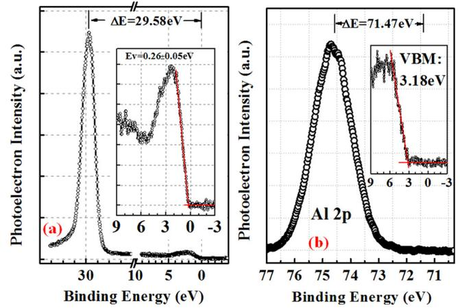
FIG. 10. XPS spectra of (a) Ge 3d core level ( $E_{\text{Ge}3d}^{\text{Ge}}$ ) and valence band maximum, VBM ( $E_{\text{VBM}}^{\text{Ge}}$ ) of (111)Ge film; (b) Al 2p core level ( $E_{\text{Al}2p}^{\text{Al}}$ ) spectrum and VBM ( $E_{\text{VBM}}^{\text{Al}}$ ) of 10 nm  $\text{Al}_2\text{O}_3$  film, respectively.
