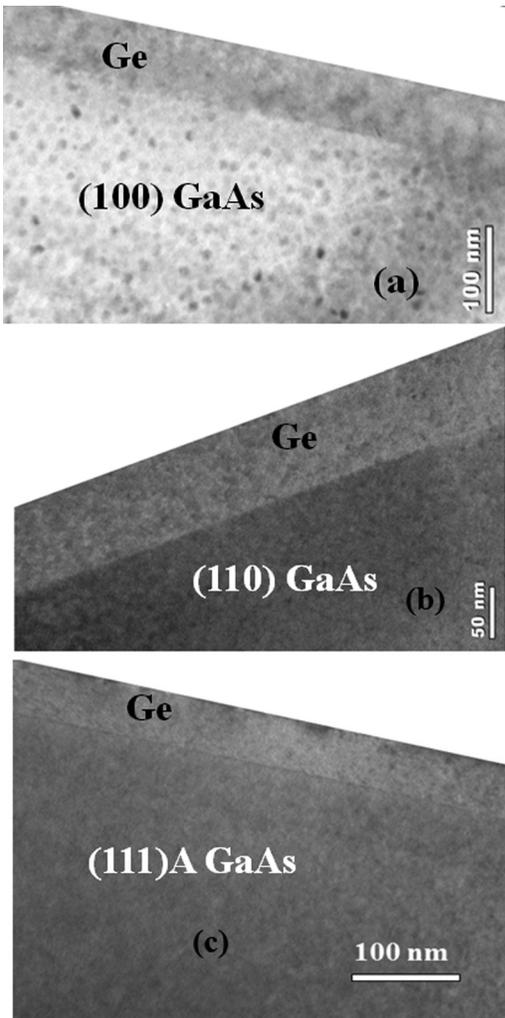
FIG. 4. Cross-sectional TEM micrograph of epitaxial Ge grown on (a) (100) $\beta$  GaAs, (b) (110) GaAs, and (c) (111)A GaAs substrates. The sharp interface between Ge and GaAs was achieved in each orientation.
