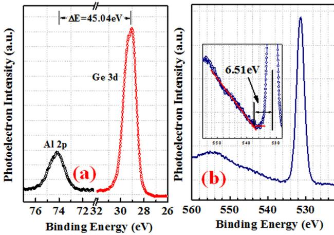
FIG. 9. XPS spectra of (a) Ge 3d ( $E_{\text{Ge}3d}^{\text{Ge}}$ ) and Al 2p core level ( $E_{\text{Al}2p}^{\text{Al}}$ ) spectra of 1 nm thin  $\text{Al}_2\text{O}_3$  film/(110)Ge interface, and (b) the CL spectrum of 10 nm  $\text{Al}_2\text{O}_3$  film. The band gap of  $\text{Al}_2\text{O}_3$  was determined to be  $6.51 \pm 0.05$  eV.
