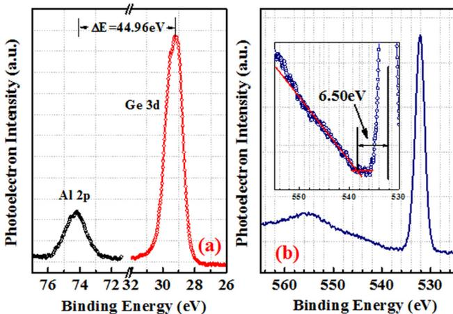
FIG. 7. XPS spectra of (a) Ge 3d ( $E_{Ge3d}^{Ge}$ ) and Al 2p core level ( $E_{Al2p}^{Al}$ ) spectra of 1 nm thin  $Al_2O_3$  film/(100)Ge interface, and (b) shows the core level spectrum of 10 nm  $Al_2O_3$  film. The band gap of  $Al_2O_3$  was determined to be  $6.5 \pm 0.05$  eV.
