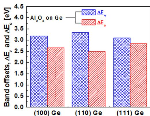
FIG. 13. Histogram of band offset distribution obtained from Al<sub>2</sub>O<sub>3</sub>/Ge heterointerface on crystallographic oriented Ge layers. The highest ΔE<sub>v</sub> value was obtained on (110)Ge.
