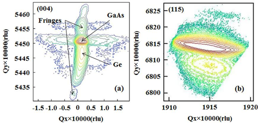
FIG. 1. (a) Symmetric (004) and (b) asymmetric (115) reciprocal space maps of 80 nm Ge/(100)GaAs ( $6^\circ$  offcut towards [110] direction) heterostructure. The RSMs are plotted in reciprocal space coordinates and each epilayer peak corresponding to reciprocal lattice point is indicated in this figure.
