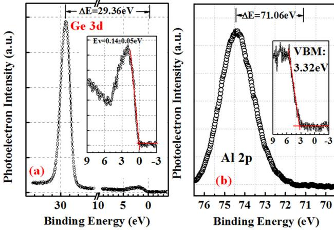
FIG. 8. XPS spectra of (a) Ge 3d core level ( $E_{\text{Ge}3d}^{\text{Ge}}$ ) and valence band maximum, VBM ( $E_{\text{VBM}}^{\text{Ge}}$ ) of (110)Ge film; (b) Al 2p core level ( $E_{\text{Al}2p}^{\text{Al}}$ ) spectrum and VBM ( $E_{\text{VBM}}^{\text{Al}}$ ) of 10 nm  $\text{Al}_2\text{O}_3$  film, respectively.
