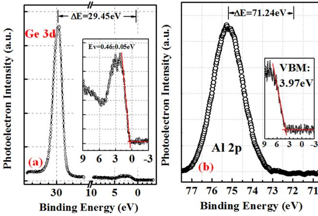
FIG. 6. XPS spectra of (a) Ge 3d core level ( $E_{Ge3d}^{Ge}$ ) and valence band maximum, VBM ( $E_{VBM}^{Ge}$ ) of (100) Ge film; (b) Al 2p core level ( $E_{Al2p}^{Al}$ ) spectrum and VBM ( $E_{VBM}^{Al}$ ) of 10 nm  $Al_2O_3$  film, respectively.
