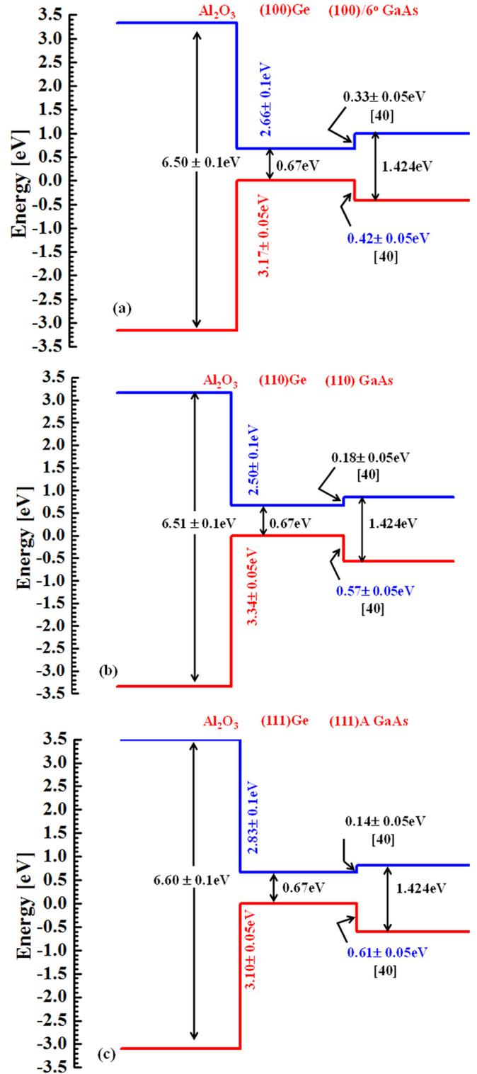
FIG. 12. Energy-band diagram of the Al<sub>2</sub>O<sub>3</sub>/Ge heterojunction obtained from XPS measurements on (a) (100)Ge, (b) (110)Ge, and (c) (111)Ge, respectively. The conduction band discontinuity,  $\Delta E_C$  has been calculated based on the measured  $\Delta E_V$  and the difference in bandgap of Al<sub>2</sub>O<sub>3</sub> and Ge, where  $\Delta E_g = \Delta E_V + \Delta E_C$ . The Ge/GaAs band offset in each orientation is included from Ref. 40.
