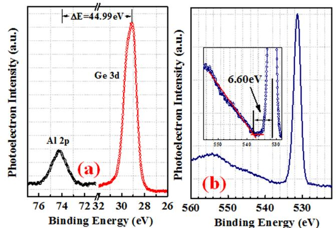
FIG. 11. XPS spectra of (a) Ge 3d ( $E_{\text{Ge}3d}^{\text{Ge}}$ ) and Al 2p core level ( $E_{\text{Al}2p}^{\text{Al}}$ ) spectra of 1 nm thin  $\text{Al}_2\text{O}_3$  film/(111)Ge interface, and (b) the CL spectrum of 10 nm  $\text{Al}_2\text{O}_3$  film. The band gap of  $\text{Al}_2\text{O}_3$  was determined to be  $6.6 \pm 0.05$  eV.
