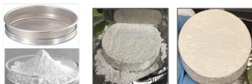
**Fig. 3.** Preparation of powder bed for quantifying bed packing density
